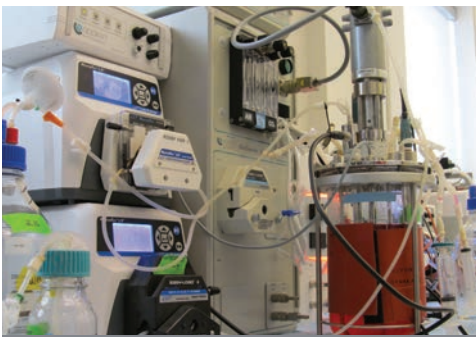
Bioreactors housed at the CCRM will enable the robust and scalable production of heart muscle cells needed for cell therapy applications. (Image credit: CCRM)
