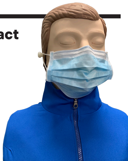
This mannequin's oral cavity was fitted with a latex balloon filled with compressed oxygen and dye to simulate a patient's cough during an eye examination
