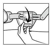
B. Lift the plastic tab off of the screw on the right side.
