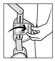
B. Lift the plastic tab off of the screw on the right side.
