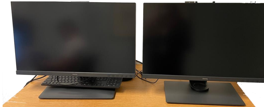
Figure 4. Devices for the present study. The screen on the left is the Flicker-Free screen, and the screen on the right is the Flicker screen. THEY LOOK THE SAME, but is one better tolerated than the other?
