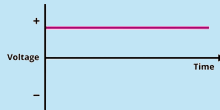
How Can a Screen be Flicker-Free? Direct Current (DC)
