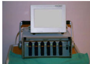
HeartMate Power Base unit
